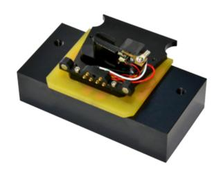
Both Z probe holders include a probe exchange guide which facilitates probe exchanges. To exchange probes, the probe module is simply placed on top of the exchange guide, light pressure is applied, the guide then releases the probe clamping spring, and the probe is then easily exchanged.
