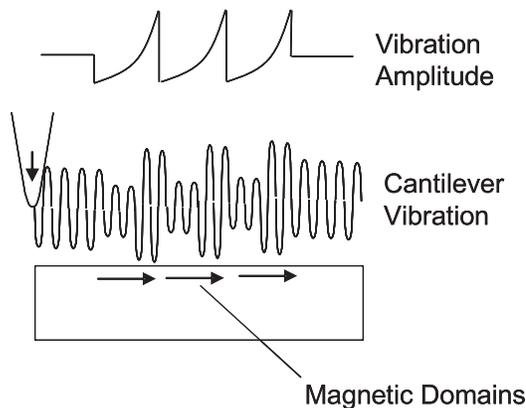
*On the second pass of the vibrating probe over the surface, the probe is raised a fixed distance from the surface. Magnetic fields from the surface cause the vibration amplitude and phase to change. The MFM image is created by displaying the changes in amplitude and/or phase.*
