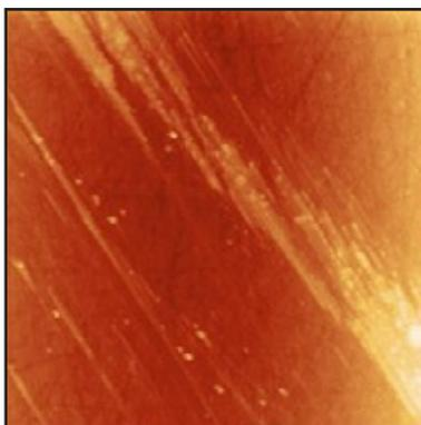
AFM image, Magnetic Read/Write Head 40 X 40  $\mu$ m
