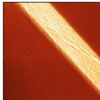
MFM image, Magnetic Read/Write Head 40 x 40  $\mu$ m
