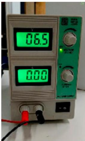
A power supply is used to directly supply a biast to the probe or the sample.
