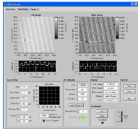
Once all the steps in the pre-scan window are completed, the scan window is used for measuring images. Scan parameter, Z feedback parameters, and image view functions may be changed with dialogs on this screen.
