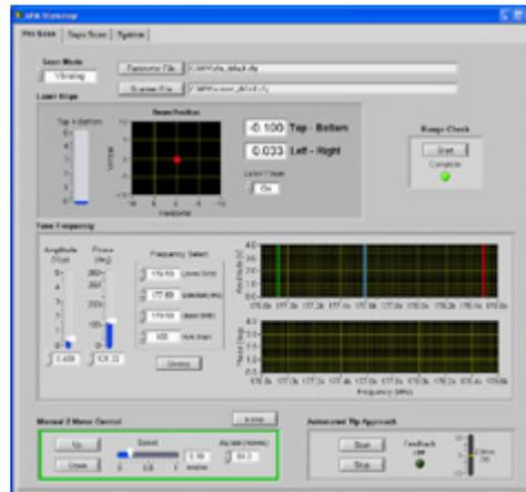
A pre-scan window includes all of the functions required before a scan is started. The functions are presented in a logical sequence on the screen.
